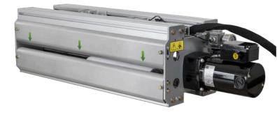
The Uni-Roller<sup>®</sup> S2 Powered lubricator uses a photo eye sensor to detect blanks and provides an input to the SPR-2000<sup>™</sup> programmable fluid controller.
