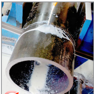
Sawing with coolant
