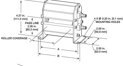
Vertical Mini-Rollers<sup>™</sup> coverage up to 4" [102 mm]
