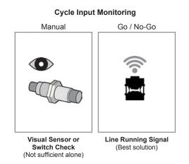
that it provides fail-safe operation: the circuit is closed when the press is not running, and the circuit is open when the press is running. Implementing this could take some programming effort and electrician time, however, the insurance it provides is well worth the cost.
