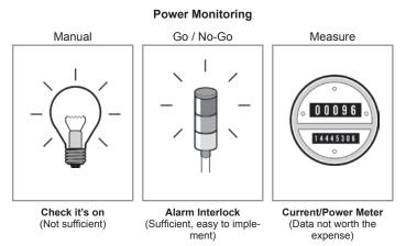
A third option would be to measure input power or electrical current to the controller system. With this third option, the manufacturer would know exactly how much electrical current the lubricator was drawing for each part stamped (knowing this information may or may not be beneficial).
