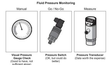
will rely on the alarm interlock relay to prevent the press from running. Consistent fluid pressure is absolutely essential to providing consistent lubrication. The flow rate of fluid to the rollers and nozzles is directly related to the pressure in the fluid tank, and knowing the exact pressure when each part was made could be quite valuable as it directly relates to the amount of lubricant applied to the stock material.
